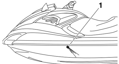
1 Cooling water pilot outlet (port [left] side)
