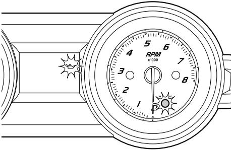
If the oil pressure warning is activated, immediately reduce the engine speed, return to shore, and then check the engine oil level. (See page 51 for information on checking the engine oil level.) If the oil level is sufficient, have a Yamaha dealer check the watercraft.
