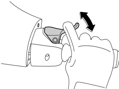
Face the handlebars straight ahead with the handlebars in the lowest position and the throttle lever in the fully closed (idle) position, and then make sure that there is the proper amount of throttle lever free play when the throttle lever is in the fully closed (idle) position. (See page 30 for telescopic steering system operation procedures.)
