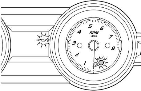
If this occurs, immediately reduce the engine speed, return to shore, and then check the engine oil level. (See page 47 for engine oil level checking procedures.) If the oil level is sufficient, have a Yamaha dealer check the watercraft.
