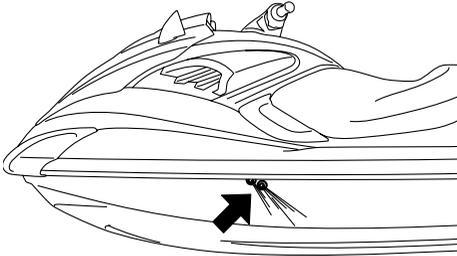
To check for proper operation of the cooling system, check that water is being discharged from the port (left) pilot outlets. If water is not being discharged from these outlets, cooling water may not be circulating in the engine. When this occurs, stop the engine and check for the cause. (See pages 38 and 85 for more information.)
