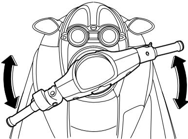
Pull the handlebars up and down to check that the lock lever and handlebars are locked in
