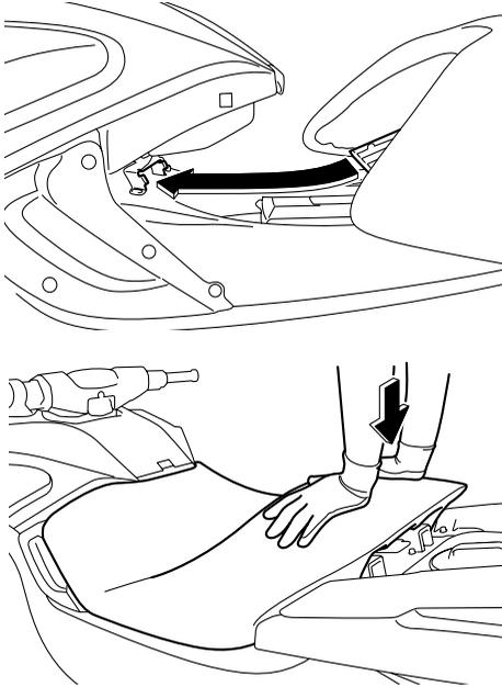
(2) Install the rear seat. Make sure that the seats are securely installed before operating the watercraft.
