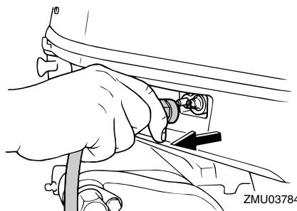
3. Press the power trim and tilt switch / power tilt switch "UP" (up) until the outboard motor has tilted up completely.
