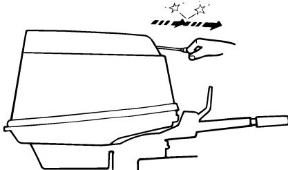
6. After the engine starts, slowly return the manual starter handle to its original position before releasing it.
