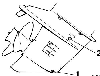
1. Gear oil drain screw
