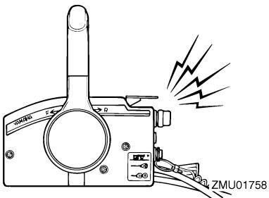
If the warning system has activated, stop the engine and check the cooling water inlet for clogging.
