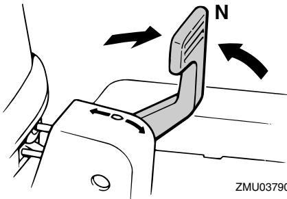
2. Push the shallow water lever down to the release position.
