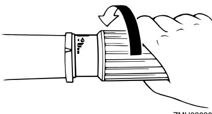
2. Move the gear shift lever quickly and firmly from neutral to forward.
