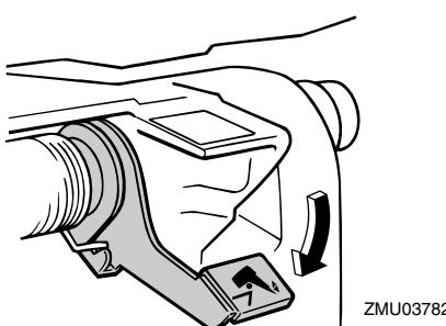
4. Hold the rear of the top cowling with one hand, tilt the engine up, and turn the tilt support lever to the lock position and support the engine.
