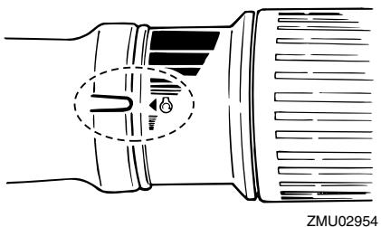
4. Pull out / turn the choke knob fully. After the engine starts, replace / return the knob to the home position.
