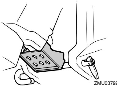
4. To return the outboard motor to the normal running position, place the gear shift lever in neutral, then slightly tilt the outboard motor up. Set the tilt lock lever and shallow water lever to the lock position and slowly tilt the outboard motor
