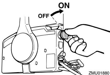
4. Open the throttle slightly without shifting using the neutral throttle lever or free accelerator. You may need to change the throttle opening slightly depending on engine temperature. After the engine starts, return the throttle to the original position.
