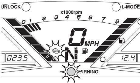
If the check engine warning is activated, immediately reduce the engine speed, return to shore, and have a Yamaha dealer check the engine.
