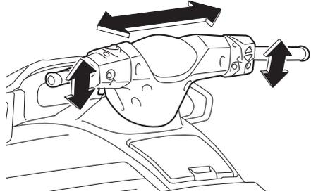
Turn the handlebars as far as possible to the right and left to make sure that the jet thrust nozzle moves as the handlebars are turned, and that there is no difference between the
