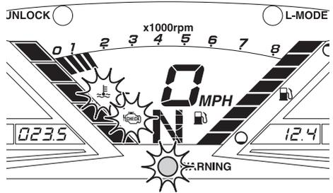
If the engine overheat warning is activated, immediately reduce the engine speed, return to shore, and then make sure that water is being discharged from the cooling water pilot outlet while the engine is running. If there is no discharge of water, stop the engine, and then check the jet intake for clogging. (See page 94 for information on the jet intake.)
