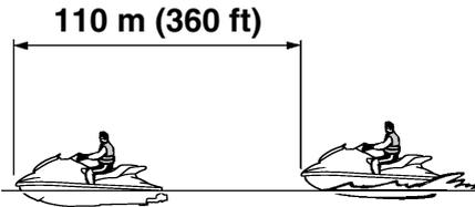
If the RiDE lever is squeezed to slow down, the stopping distance is approximately 30% shorter than when the RiDE lever is not used. However, this distance will vary depending on many factors, including gross weight, water surface conditions, and wind direction.
