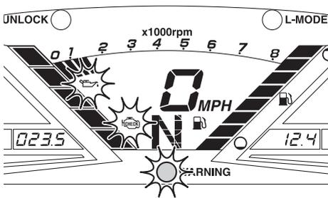
If the oil pressure warning is activated, immediately reduce the engine speed, return to shore, and then check the engine oil level. (See page 52 for information on checking the engine oil level.) If the oil level is sufficient, have a Yamaha dealer check the watercraft.
