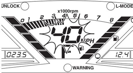
sound one time quickly and the set engine speed will change. However, the adjustment is limited to a maximum of five increments above or below the initial cruise assist setting.
